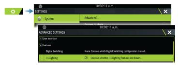
Once the ITC lighting controller is installed and connected to the NMEA 2000<sup>®</sup> network, it should appear in the control bar. If it is not appearing in the control bar, you can activate it from the Advanced settings dialog.
