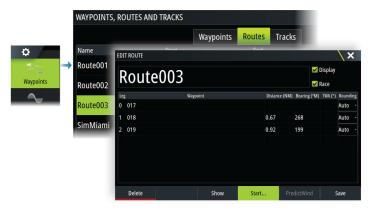
When route navigation is viewed, the menu expands and shows options for canceling the navigation, for skipping a waypoint, and for restarting the route from current vessel position.
