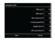
This option allows for manually changing parameters that were set during the commissioning of the autopilot computer. For more details of the settings, refer to the separate documentation for the autopilot computer.
