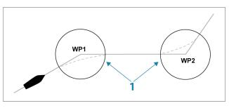
The arrival circle (1) should be adjusted according to boat speed. The higher the speed, the wider the circle.
