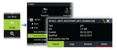
• From the forecast menu option on the chart panel. The Grib weather option is only available if Grib weather is set as the overlay on the chart.
