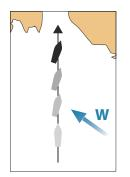
In NAV mode the autopilot automatically steers the vessel to a specific waypoint location, or along a pre-defined route. Position information is used to change the course to steer to keep the vessel on the track line to the destination waypoint.
