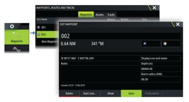
When navigating to a waypoint, the menu expands and shows options for canceling and for restarting the navigation from current vessel position.
