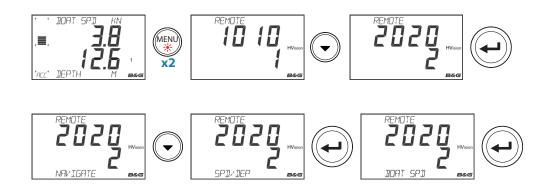
Use the **UP/DOWN** and **ENTER** keys to navigate to a variable and select the variable to display. Exit by pressing the **PAGE** key.
