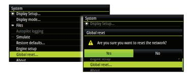
→ **Note:** After performing a global reset the Graphic Display will ask to do an auto source selection. A global reset will reset all system modules and devices back to default settings and will need to be re-configured before use.
