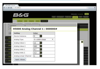
→ **Note:** The recommend calibration procedure for a positional sensor (i.e. Boom Angle, Rudder Angle, Keel Angle etc.) is to move the sensor to its maximum Starboard positon, pressing the
