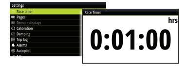
→ **Note:** The timer set value is in Hours: Minutes (hh:mm), the timer counter will show Minutes: Seconds (mm:ss) with the hours shown in the top right hand corner of the display.
