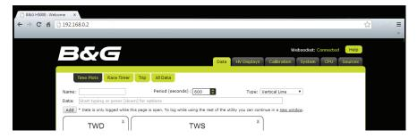
→ **Note:** It will say "Websocket: Connected" in the top right-hand corner of the screen next to the help tab. If it says "Websocket: Not Connected" then check the CPU and router power and connections.
