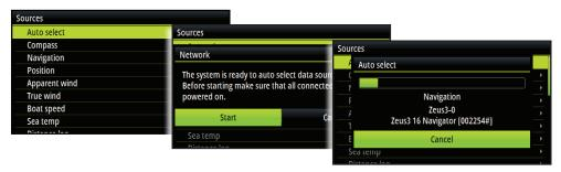
The operator will be informed when the auto select process is completed.
