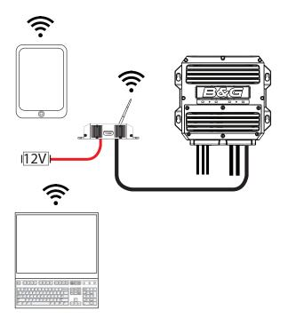
→ **Note:** To connect the WiFi-1 router to the H5000 CPU an Ethernet to RJ45 converter cable is required.
