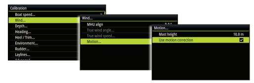
→ **Note:** A 3D Motion sensor and mast height value is required in conjunction with a CPU running Hercules level software or greater to use this feature.
